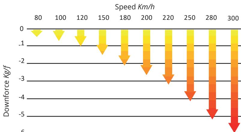
The Downforce that the spoilers generates raises potentially as the speed increases, at 300 km/h we get 5,8 Kg/f.
