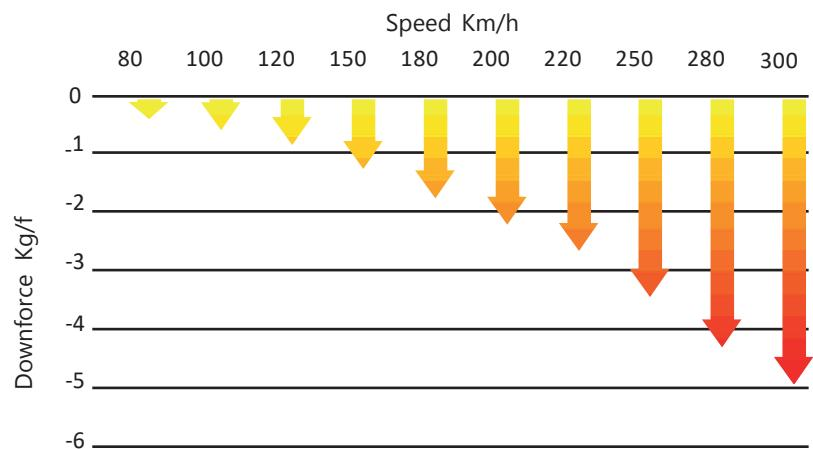
The Downforce that the spoilers generates raises potentially as the speed increases, at 300 km/h we get 4.9 Kg/f.
