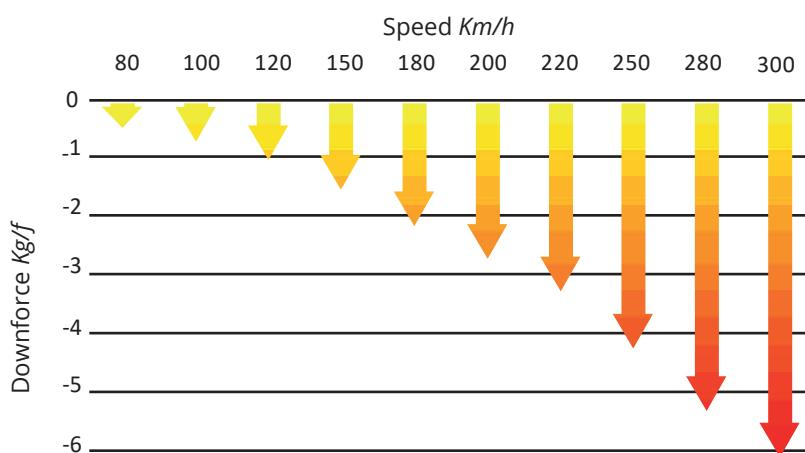
The Downforce that the spoilers generates raises potentially as the speed increases, at 300 km/h we get 6,2 Kg/f.
